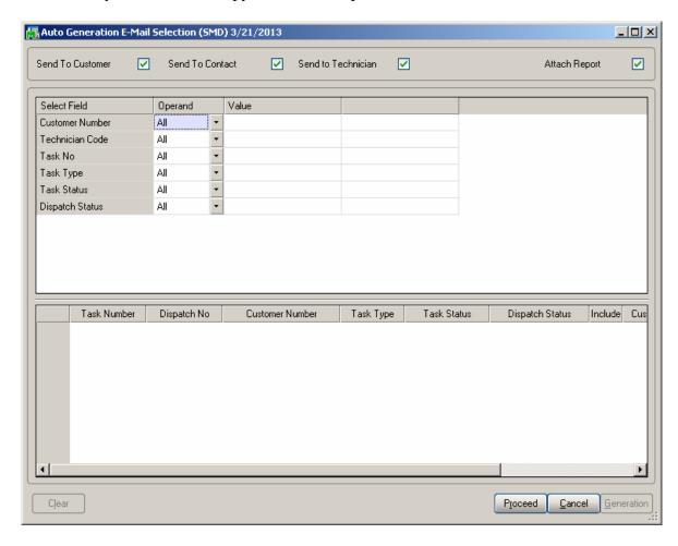
You can choose to process all the customers, technicians and tasks or select only those with codes falling into the range set by starting and ending. Also you can select tasks and dispatches by Type and Status.
