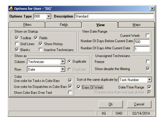
Check the corresponding boxes in the **Show on Startup** section to show **Toolbar**, **Grid Lines**, **Fields**, **Blanks**, **History**, **Inactive Technicians** each time the Dispatch Board starts. The **Show History** option enables displaying **Closed** tasks (with their dispatches) on the Dispatch Board.
