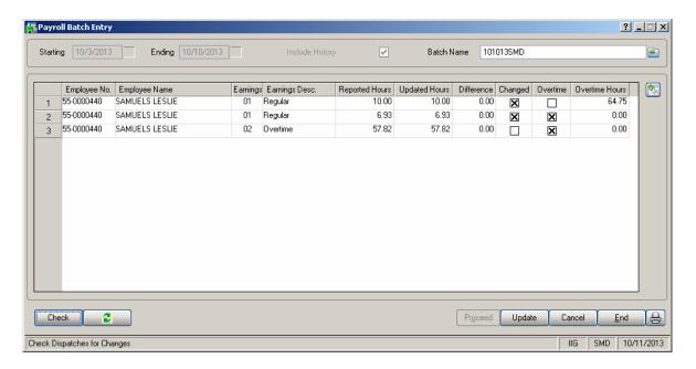
For a previously entered batch, click the **Check** button to find out if the Labor lines in dispatches have been changed, added or removed since the entry of the batch.
