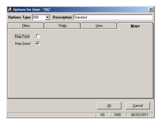
Select the **Map Quest** checkbox to enable Map Quest for Dispatch Board. The Dispatch Board integration with Map Quest allows the users to enter a region, specify date range and display on the map-board the technicians in the filtered region for the specified date(s).
