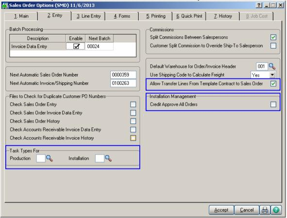
The **Task Types for** options allow specifying Task types to be used when generating Task for Sales Order Header.
