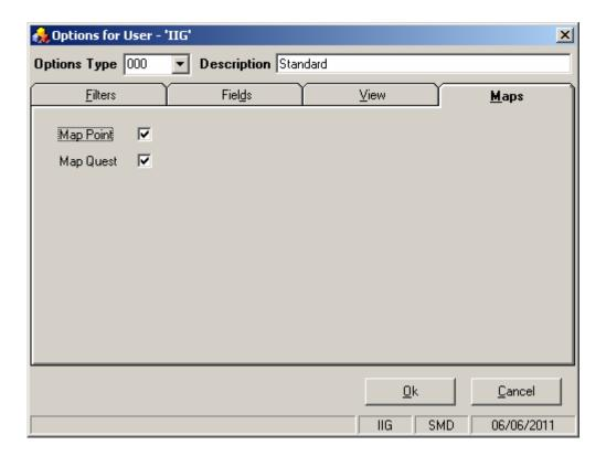
**Map Point** and **Map Quest** fields become enabled after installing correspondingly SMM4.50 and SMQ4.50 enhancements.
