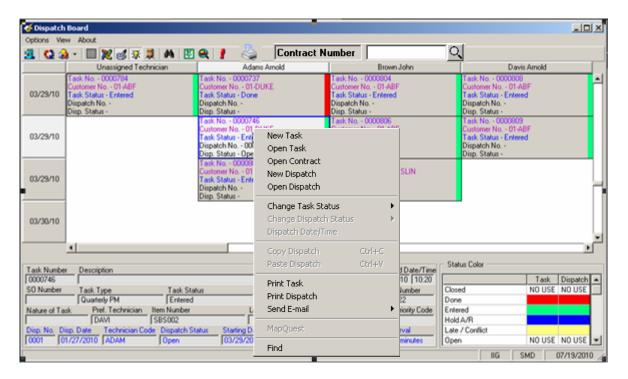
**New Task-** opens the **Task Data Entry** screen ready for new task entry. The **Next Task Number** is selected, and the **Scheduled Date/Time** is set equal to the selected cell **Date/Time**. The selected cell **Technician** is loaded after selecting the **Customer**.
