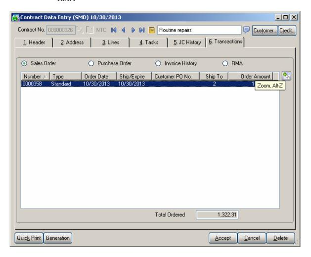
The Zoom button on the right hand of the list box enables drill down to the selected entry.
