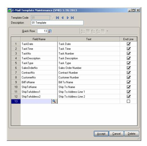
For the selected **Template Code**, select which fields value you want to add to the current line from the **Field** drop-down list. If you haven't entered Text for that field yet, clicking in the **Text** field will bring the name of the selected Field, which you can edit then. You can add lines containing only Field (no Text), only Text (no Field), or completely empty lines.
