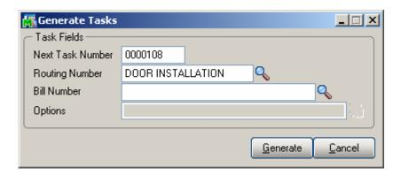
When the **Routing Number** is specified, tasks are generated for those steps of that routing, which have the **Generate Task** checked in the **Routing Maintenance**. Here are the Tasks generated for the selected Routing number:
