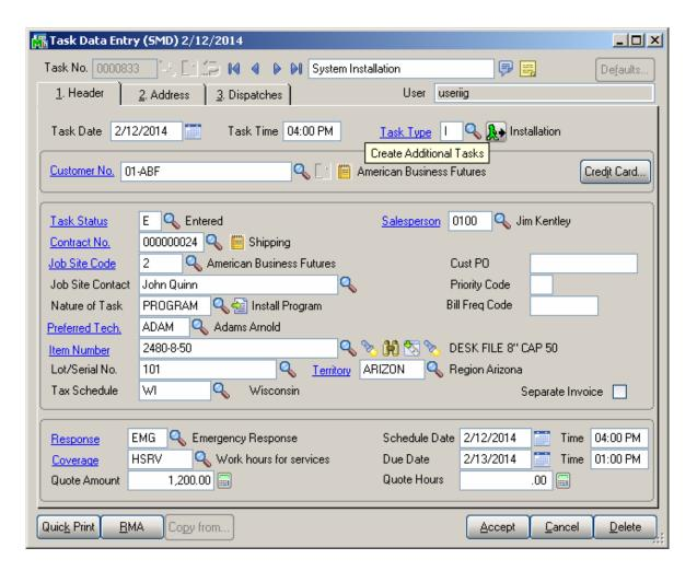
If the task is of a type, for which the **Create Additional Task** box is checked in the **Task Type Maintenance**, the Create Additional Tasks button become enabled allowing the user to automatically generate additional tasks.
