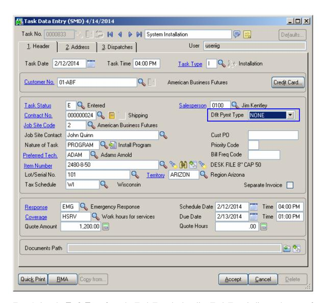
Enter/select the **Task Type** from the Task Type lookup list. Task Type indicates the type of the task to be performed. It is a required field for Task Entry.
