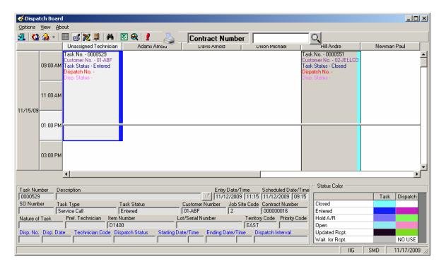
The **Status Color** legend in the lower right hand corner next to the Task/Dispatch data displays the colors specified for corresponding Task/Dispatch statuses.
