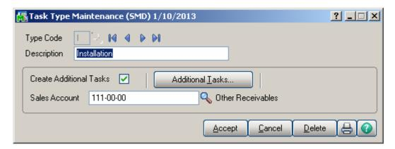
**Sales Acct** is used for postings when closing dispatches with labor (based on the priority in **Service Management Options**).
